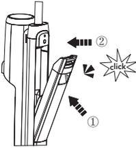
Place the tank back into the appliance. You should hear a "Click" if done correctly.
