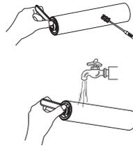
Using the cleaning tool, remove the hair and debris wrapped around the roller and rinse with water. Replace the brush roller back into the accessory holder, and allow it to dry completely before reinstalling.
