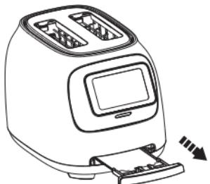
To clean any crumbs from the toaster, remove the crumb tray by pulling it outwards. Replace the crumb tray by sliding it inwards until it locks into position. And empty the crumb tray before using the toaster again.
