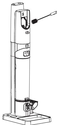
Clean air channel with cleaning tool when the air channel is blocked, pull out the dustbin for cleaning.
