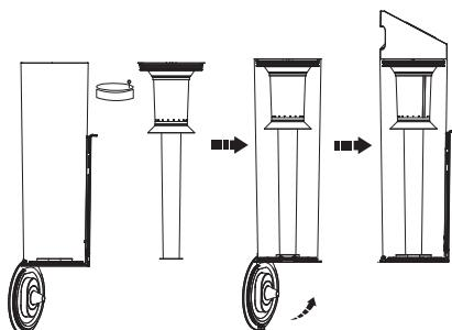
After cleaning, install the mesh filter dustbin back into the Clean Station.
