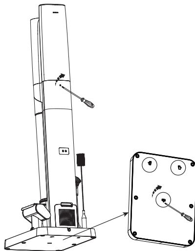
In the event that the Clean Station needs to be disassembled, press the latch with tool to remove the three parts.
