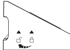
Turn counter-clockwise to open the upper cover, and then remove the filter cotton and filter element.
