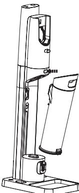
Press the release button and pull outward to remove the dustbin.
