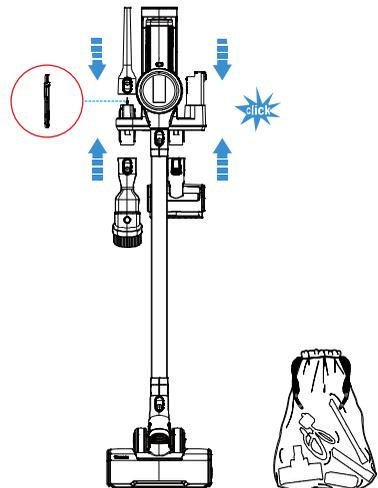
To avoid the deformation of the bristles, always put away the accessories on the docking station after use, a 'click' sound will be heard when it has been successfully accomplished. The rest parts can be stored in the tools bag.
