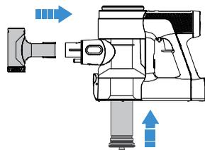
Replace a clean filter to the main body. Put the dirty pre-filter into the cleaning tool and connect the cleaning tool to the main body.
