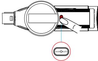
In AUTO mode, press the MAX/AUTO button and switches to Max mode.
