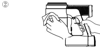
Clean with wet cloth. Do not allow water to enter the appliance, especially not into motor and battery.
