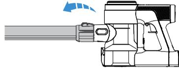
Press the release button and remove tube.
