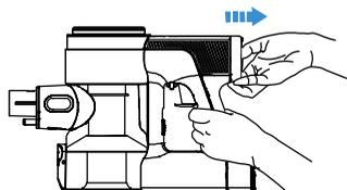
Press the HEPA release button and gently pull out the HEPA to remove the dust.
