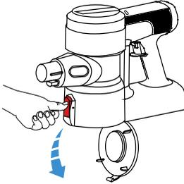
When finished, press the release button on the side of the dustbin and empty the contents.
