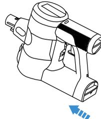
Slide the battery into the bottom of the main body. The battery will click into position when correctly fitted.
