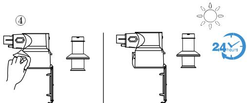
Clean the dustbin and mesh filter with wet cloth. The two parts should be air dried completely before reinstalling.
