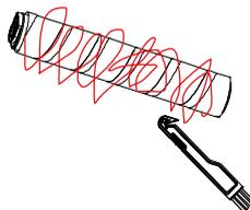
Remove the hair and debris wrapped around the roller with Tineco Hair Cleaning Tool.
