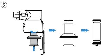
Twist anti-clockwise and remove the filters.
