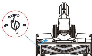
Use a coin or other tool, to unlock the brush roller lock, then remove the brush from the brush window.
