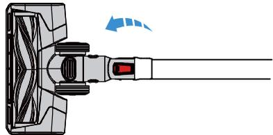
Press the release button and remove power brush.
