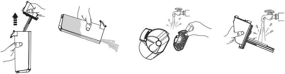
If the Dirty Water Tank lid and the filter inside have been blocked, remove the tank lid and the filter, rinse both parts with water.
