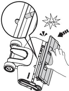
While replacing, always latch the brush cover into place to avoid leakage.
