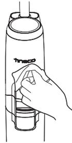
Use a cloth to clean the surface with a neutral detergent. The cloth should be dry to prevent water from entering the appliance.
