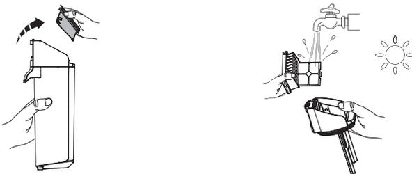
Grasp recessed area on each side of the dry filter and pull upward. Rinse under running water and must be completely dry before recombining with the lid of the DWT.
