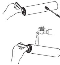
Use the cleaning tool to remove the hair and debris wrapped around the roller and then rinse the roller with water. Replace the brush roller back into the accessory holder, and allow it to dry completely before reinstalling.
