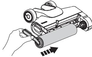
Replace the brush roller by inserting the brush roller end into the right side of the holder, then attach the roller tab to the magnetic buckle on the left side to lock into place.
