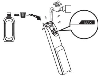
Open the tank cap, and fill with tap water to the Max line. When deep cleaning is necessary, add one bottle cap of solution to the CWT and tightly close the cap.
