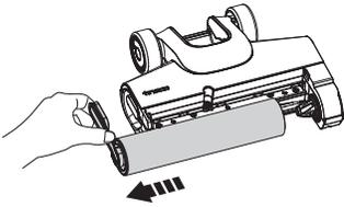
Remove the brush roller by grabbing the brush roller tab and pulling out.
