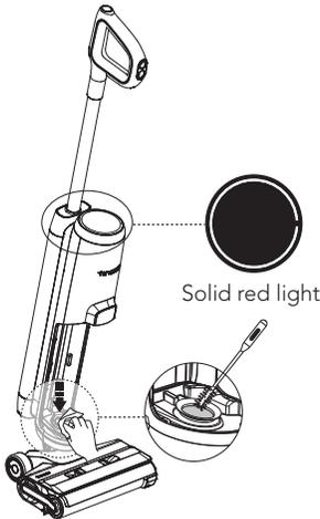
When LED loop illuminates red, remove Dirty Water Tank, clean the dirt sensor with a damp cloth or the cleaning tool.
