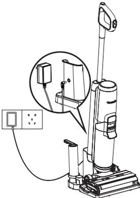
To charge the appliance, place the appliance on the charging dock and plug the adaptor into a power outlet.
